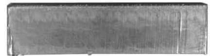
Cuts made with natural gas are cleaner with little slag and require much less grinding
